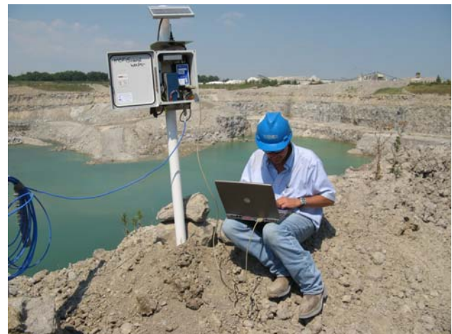
A TROLL Link Telemetry system communicates with remotely deployed monitoring equipment and allows operators to view and acquire data without site visits.
